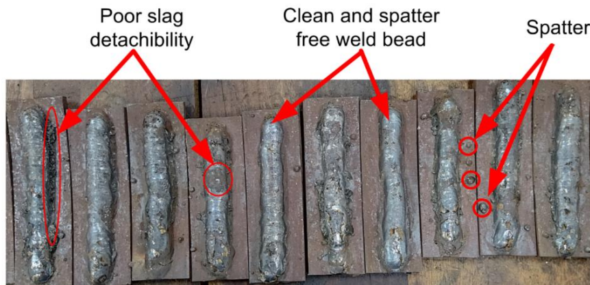
Figure 5.11: Visual inspection of bead on plate specimens
