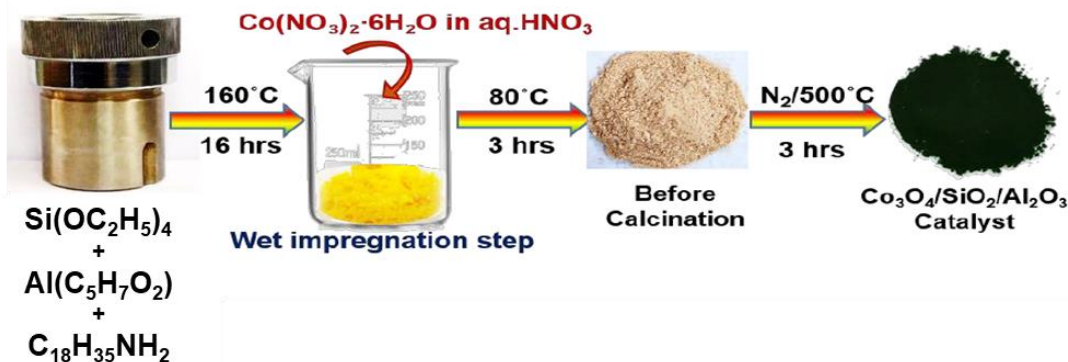
Figure 4.1 Schematic illustration of cobalt oxide loaded silica-alumina heterogeneous catalyst synthesis.
