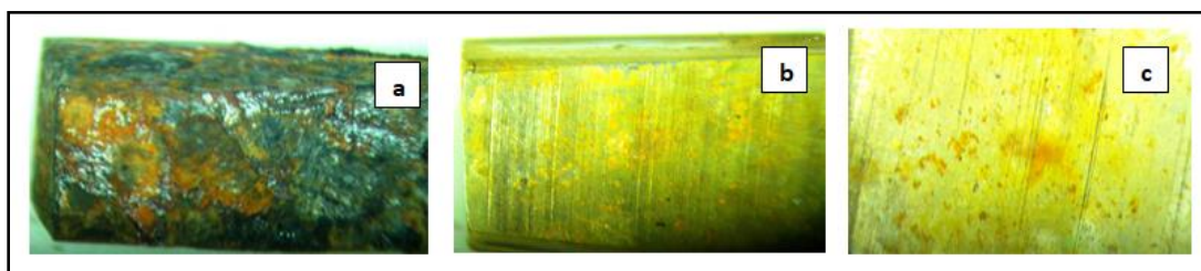
Figure 5.80: Corroded specimens in 3.5% NaCl solution (a) X70 steel (b) As Received SDSS (c) 875-180 SDSS
