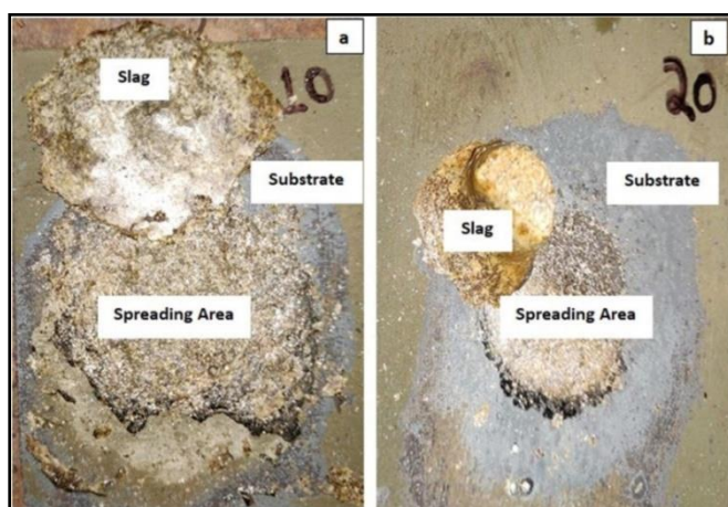
Figure 5.4: Types of melting and spreading patterns: (a) Complete melting (b) Partial Melting
