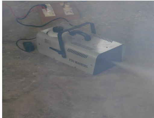
Figure 7.9: Fog machine for smoke generation in tank decoy
