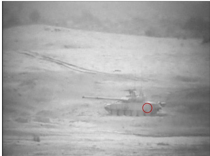
Figure 7.8 : Thermal imagery of Exhaust smoke emission of real Tank
