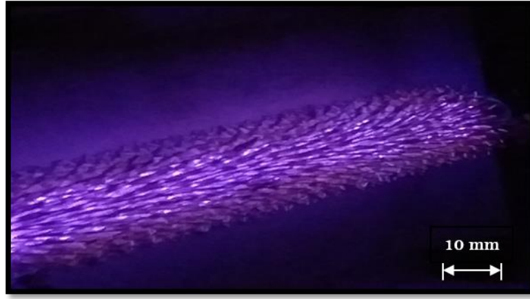
Figure 3.1: Original view of the coaxial DBD plasma device.
